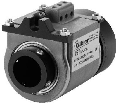
The SR060 is a compact, economical slip ring for up to 3 power and 2 signal transmissions from a stationary to a rotating platform.
